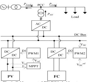
Fig. 1. Grid-connected PV-FC hybrid system.
