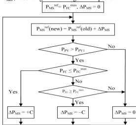
Fig. 5. Control algorithm in the UPC mode ( P<sup>ref</sup><sub>MS</sub> automatically changing)
