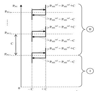
Fig. 6. Hysteresis control scheme for P<sub>MS</sub><sup>ref</sup> control.
